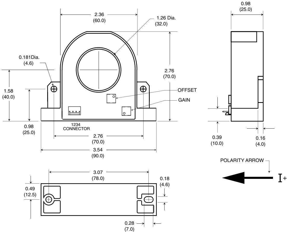
Mating Connector: Molex: Terminal 08-50-0114 (4 pieces), Connector 22-01-2047 (1 piece)
